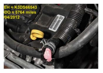
Also, if OAT-type coolant is mixed with HOAT-type coolant at greater than 95/5 ratio, corrosion inhibition will be severely reduced or eliminated. That means if one of your technicians adds the wrong coolant type to a customer's vehicle — it will be very expensive to resolve and may require replacing the engine.
